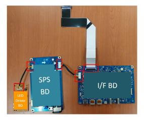
**S18** Remove electrolyte capacitors (red mark) from printed circuit boards
