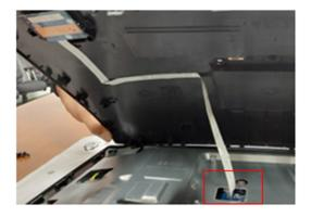
**S5** Tear off the tapes from CTRL BD FFC on Rear Cover
